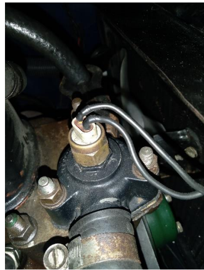
Thermostat cover with fan Switch in place
