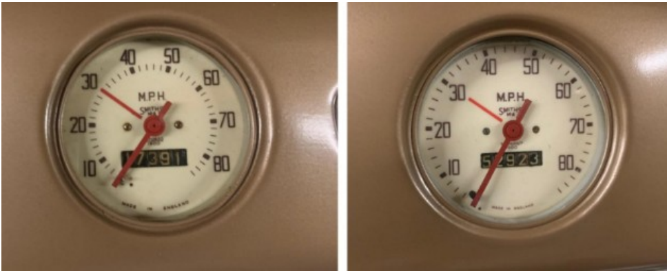
Figure 5: Two Morrie speedos - Early MM style, on left, and later MM and Series 2 style, on right
