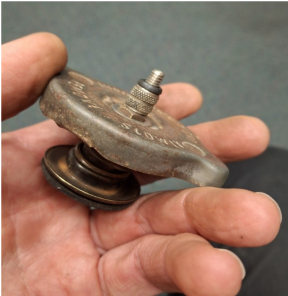
The radiator cap adapted for pressurising the radiator. The British-style bicycle valve stem comes out the top...
