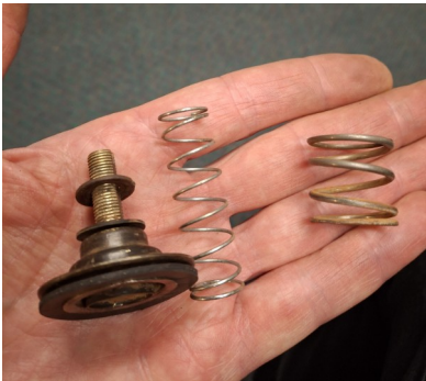
I added a second spring inside the main spring for extra pressure
