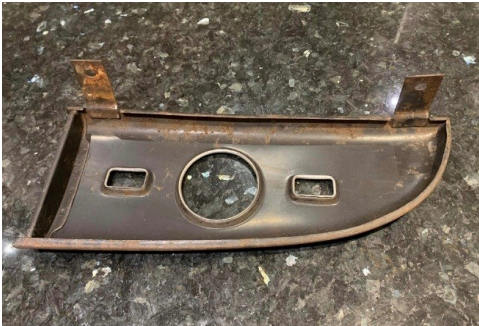
Figure 7: Later-style instrument panel with welded brackets on bottom rim
