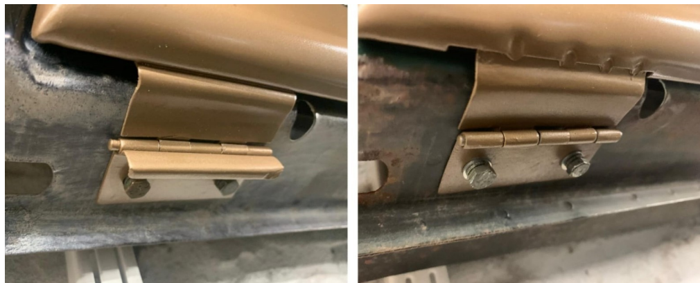
Figure 8: Change to glovebox hinge stopper--early style on left, later style on right
