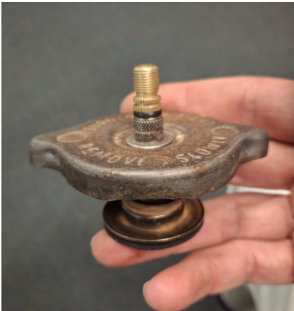
... and now with an adapter to match normal pressure hose fittings!
