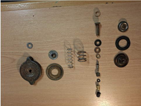
Components of the coolant system pressure tester. Note threaded bicycle valve stem.
